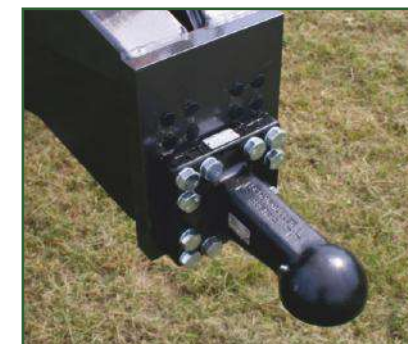
STR-505 Boltfestet kulehengerfeste, type Scharmuller, 80 mm diameter.
