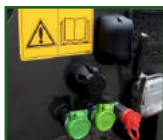
STR-1039 Rear mounted light connection 7-pin socket.
