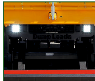
STR-1037 Two super-bright LED working lights at the rear of the trailer.
