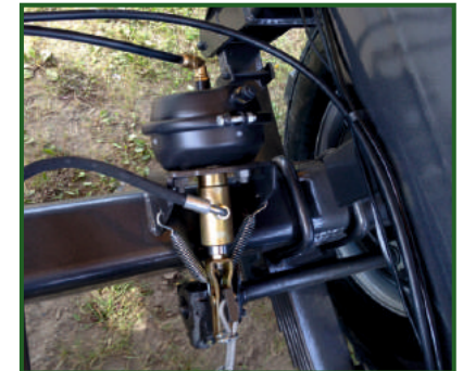
STR-305 Dual air and hydraulic brake system.
