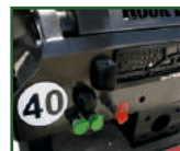
STR-1038 Rear mounted hydraulic brake connection.
