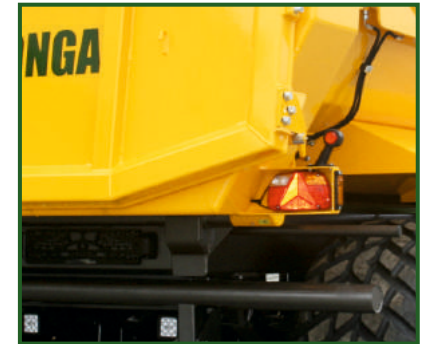
12 V electric system. Sealed loom. All lights super-bright LED.
