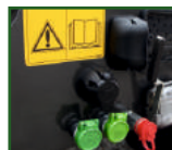
STR-1039 Rear mounted light connection 7-pin socket.
