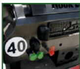
STR-1038 Rear mounted hydraulic brake connection.
