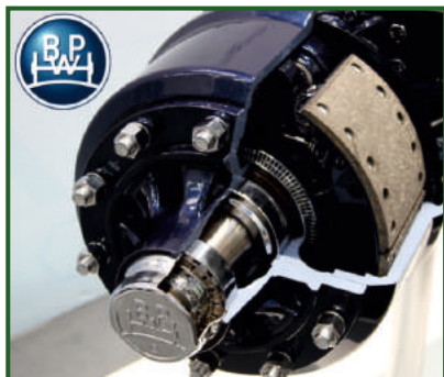
BPW commercial axle, 410x180 brake axles, 150x150 - 16mm square beam, 10 stud.
