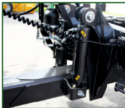
STR-508 Hydraulic drawbar for easy levelling and high comfort.
