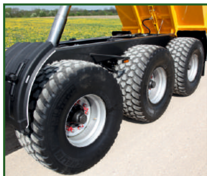
Hard plastic quarter mudguards, front and rear of the trailer.
