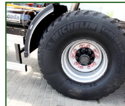
600/55 R26,5 Michelin CargoXBib radial tyres. Load rating per tyre: 7000 kg @ 40 km/h 5150 kg @ 65 km/h
