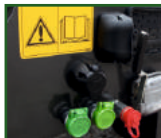
STR-1039 Rear mounted light connection 7-pin socket.
