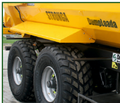
Bolted on metal mudguards.
