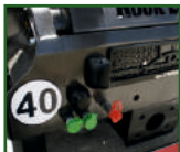
STR-1038 Rear mounted hydraulic brake connection.
