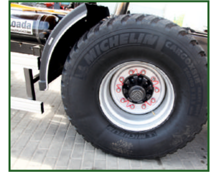
600/55 R26,5 Michelin CargoXBib radial tyres. Load rating per tyre: 7000 kg @ 40 km/h 5150 kg @ 65 km/h
