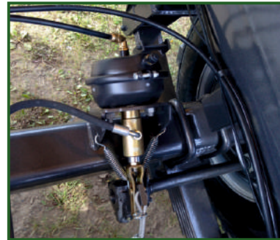
STR-305 Dual air and hydraulic brake system.
