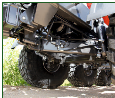
STR-410 Hydraulic suspension for optimum axle travel.
