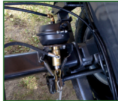
STR-305 Dual air and hydraulic brake system.
