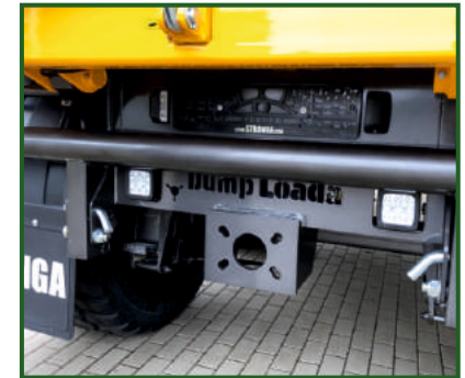
STR-1002 Rear towing eyelet mounting plate for VBG rear drawbar.
