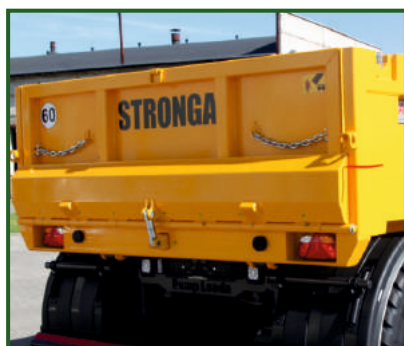
Single top-hung rear door with hydraulic flip back.
