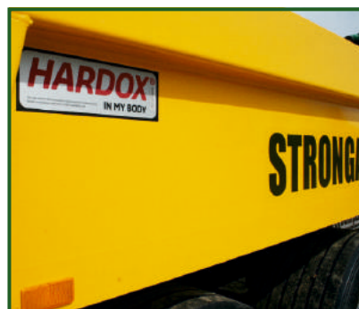
HARDOX 450 steel. 6mm floor. 4mm sides.
