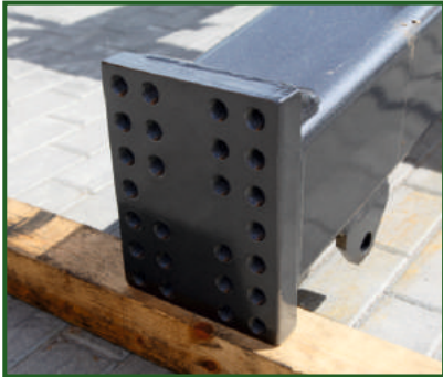
3 position plate for bolting towing eyelet.
