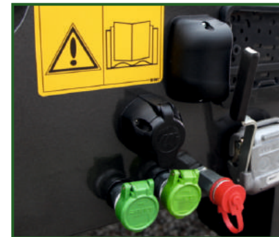
STR-1039 Rear mounted light connection 7-pin socket.
