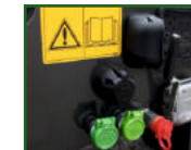
STR-1039 Rear mounted light connection 7-pin socket.
