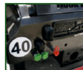
STR-1038 Rear mounted hydraulic brake connection.
