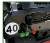
STR-1038 Rear mounted hydraulic brake connection.
