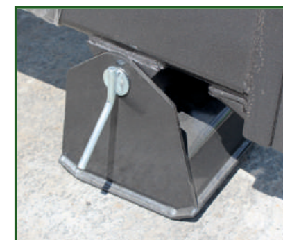
Suspended drawbar shoe with stowage point.
