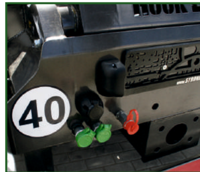
STR-1038 Rear mounted hydraulic brake connection.
