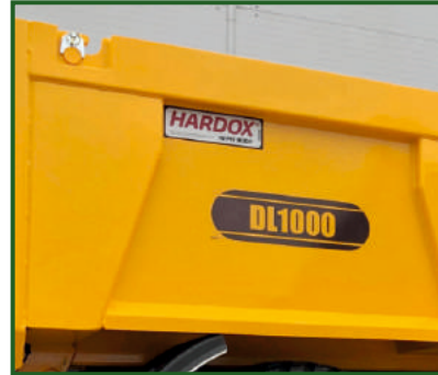
HARDOX 450 steel. 8mm floor. 6mm sides.
