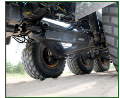
STR-410 Hydraulic suspension for optimum axle travel.
