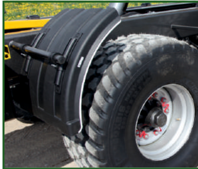
STR-903 Hard plastic quarter mudguards, front and rear of the trailer.
