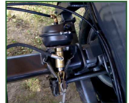
STR-305 Dual air and hydraulic brake system.
