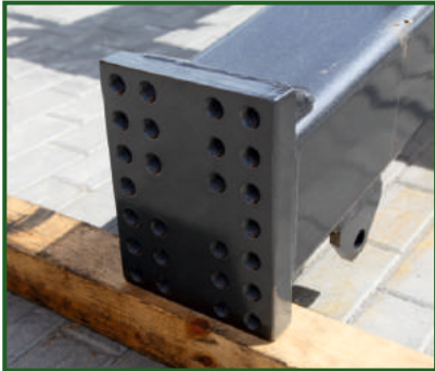
3 position plate for bolting towing eyelet.
