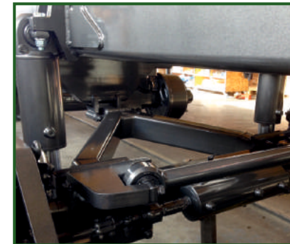
STR-410 Hydraulic suspension for optimum axle travel.
