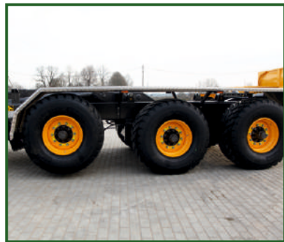
STR-411 Front lift axle - Only with air or hydraulic trailer suspensions.
