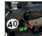
STR-1038 Rear mounted hydraulic brake connection.
