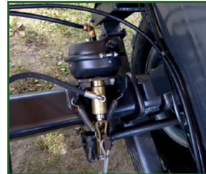
STR-305 Dual air and hydraulic brake system.
