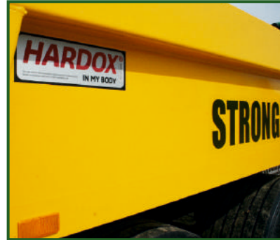
HARDOX 450 steel. 6mm floor. 4mm sides.
