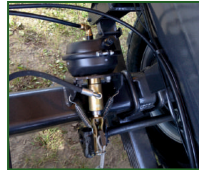
STR-305 Dual air and hydraulic brake system.
