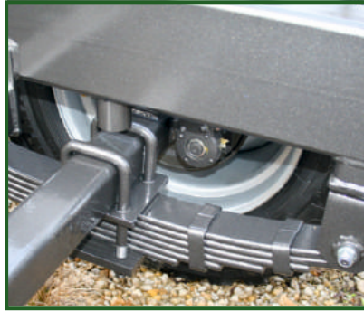
21t multileaf sprung suspension. 1480mm distance between axles.
