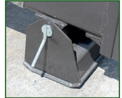
Suspended drawbar shoe with stowage point.
