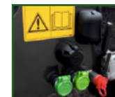
STR-1039 Rear mounted light connection 7-pin socket.
