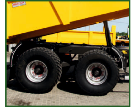
445/65 R22,5 radial tyres. Load rating per tyre: 7000 kg @ 105 km/h
