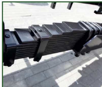
Multi-position sprung drawbar for high comfort at speed.
