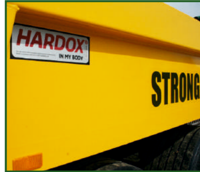
HARDOX 450 steel. 10mm floor. 8mm sides.
